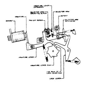
Fig. 14 - Selecting Mechanism Equipped with Holding Magnet
