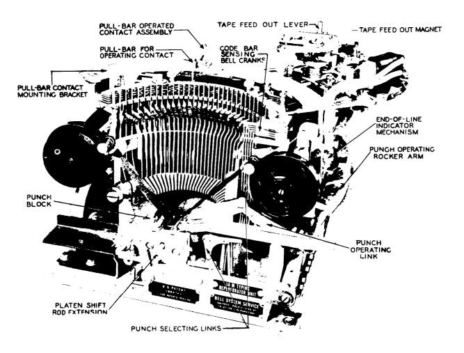
Fig. 18 - No. 14 Typing Reperforator Unit (Receiving Only - Cover Removed)
