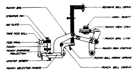
Fig. 21 - Tape Reperforating Mechanism
