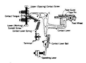
Fig. 24 - Contact Mechanism of Transmitter-Distributor
