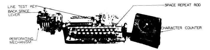
Fig. 15A - 15-Type Perforator-Transmitter
