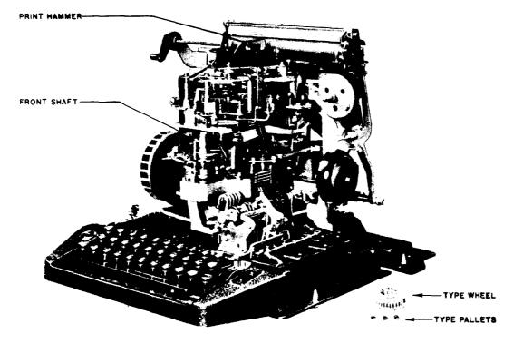
Fig. 33 - No. 26-Type Teletypewriter (Cover Removed)
