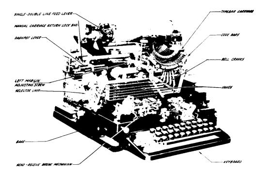
Fig. 13 - 15-Type Sending-Receiving Teletypewriter (Cover Removed)
