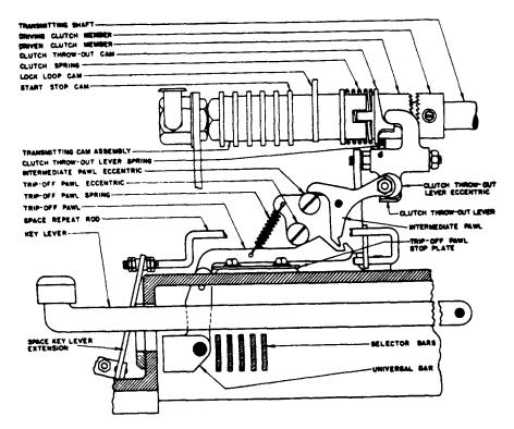
Fig. 2 - Transmitting Cam Assembly
