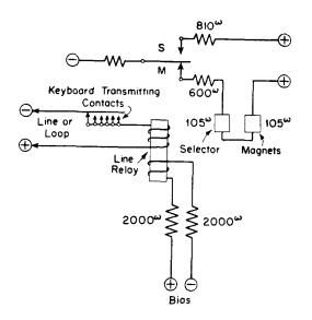
Fig. 6 - Simplified Wiring of a Teletypewriter for Neutral Operation with Line Relay
