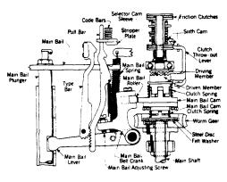
Fig. 11 - Typical Typing Mechanism
