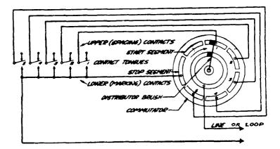
Fig. 23 - Wiring of Transmitter-Distributor Commutator and Contacts
