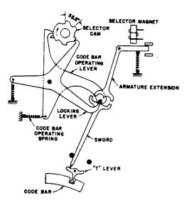
Fig. 9 - Teletypewriter Selector Mechanism Illustrating Operation of Locking Lever
