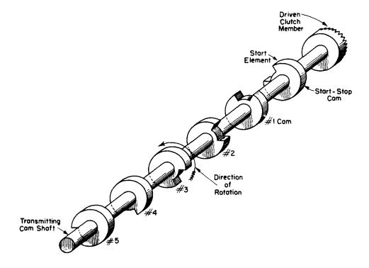
Fig. 4 - Exploded View of Keyboard Cam Sleeve Assembly
