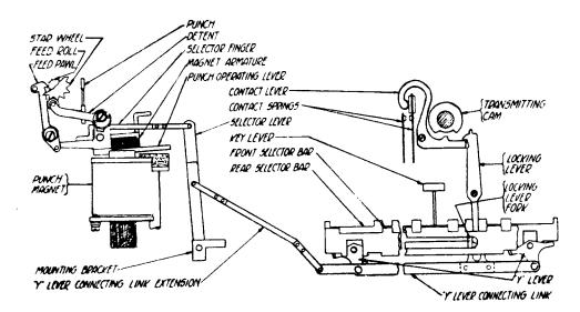
Fig. 15B - Perforator **Operating M**echanism of the 15-Type Perforator-**Transmitte**r
