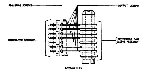
Fig. 31 - Distributor Contact Assembly - Reperforator-Transmitter
