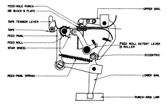
Fig. 30 - Feed-Hole Prepunch Mechanism
