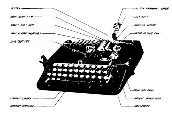
Fig. 5 - Keyboard of a 15-Type Teletypewriter
