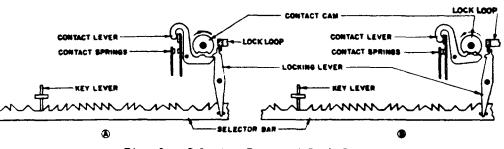
Fig. 3 - Selector Bars and Lock Levers
