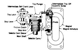
Fig. 7 - Start-Stop Arrangement of Receiving Mechanism
