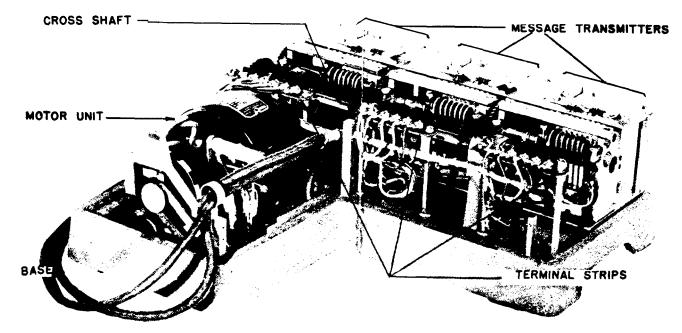
Fig. 27 - Multiple Transmitter (Cover Removed)
