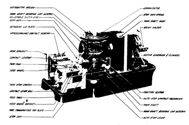
Fig. 22 - Transmitter-Distributor (Cover Removed)
