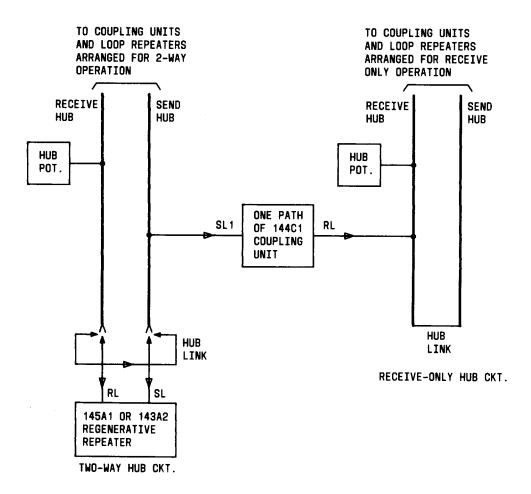
Fig. 2—Connection of Two-Way Hub Circuit to Receive—Only Hub Circuit
