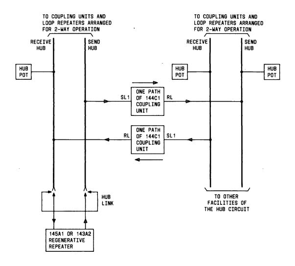
Fig. 3—Interconnection of Two-Way Hub Circuits
