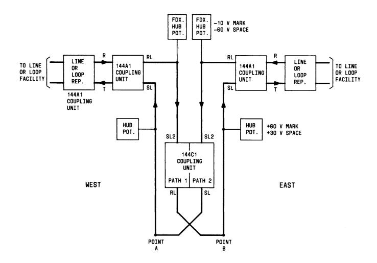
Fig. 4—144C1 Coupling Unit Arranged for Full-Duplex Service in Conjunction with 144A1 Coupling Units
