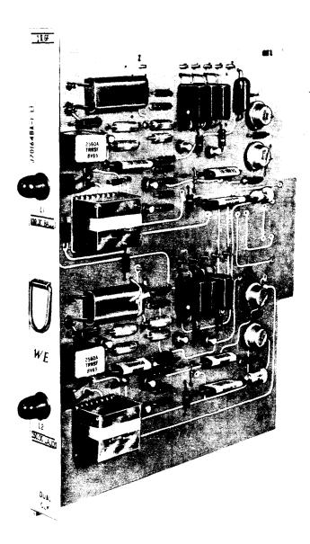
Fig. 6 — J70164BA 145A1 Regenerative Repeater Dual Clock Printed Wiring Board Unit
