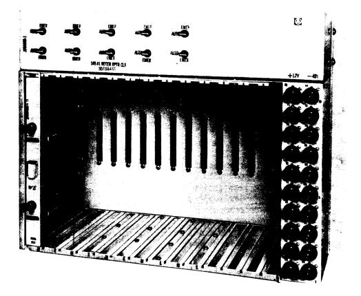
Fig. 2 — J70164B 145A1 Regenerative Repeater Dual Clock Unit Housing (Front View)
