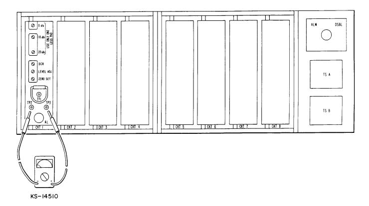
Fig. 1—Typical Method for Making Level Adjust Measurements
