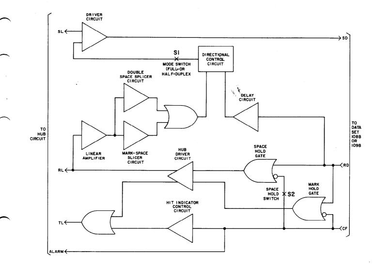
Fig. 4—Data Auxiliary Set 811C, Functional Block Diagram
