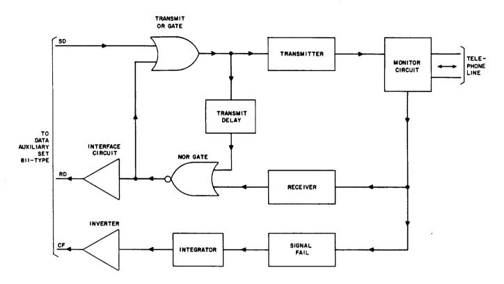
Fig. 6—Data Set 109B Functional Block Diagram
