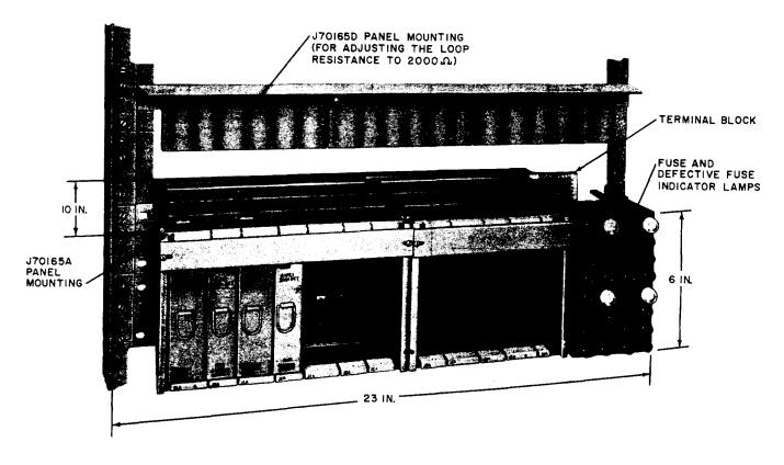
Fig. 5—Data Set 109B-Type and Data Auxiliary Set 811C Installed in Panel J70165A With Attached J70165D Panel
