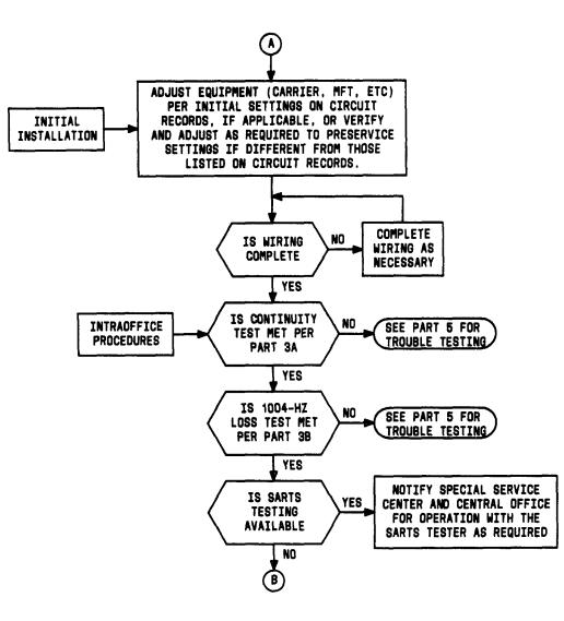
Flowchart 1—Required Preservice and Trouble Tests (Sheet 2 of 7)
