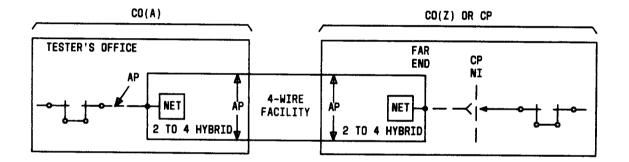
Fig. 3—2-Wire to 4-Wire Conversion at Both Ends
