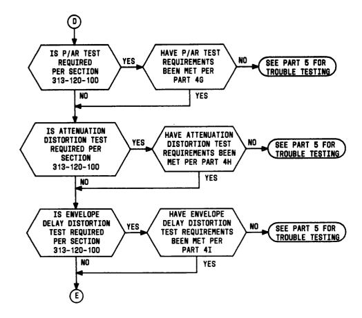
Flowchart 1—Required Preservice and Trouble Tests (Sheet 5 of 7)
