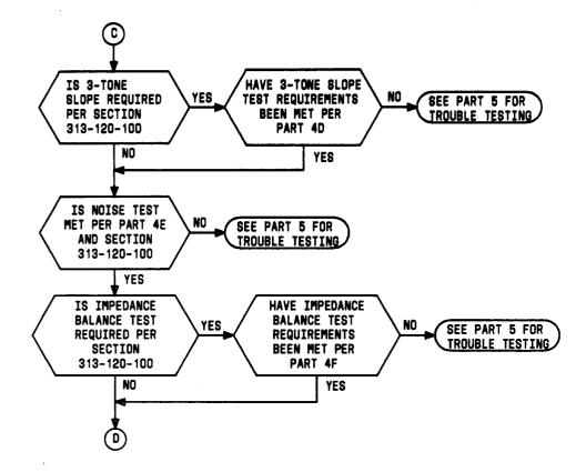
Flowchart 1—Required Preservice and Trouble Tests (Sheet 4 of 7)
