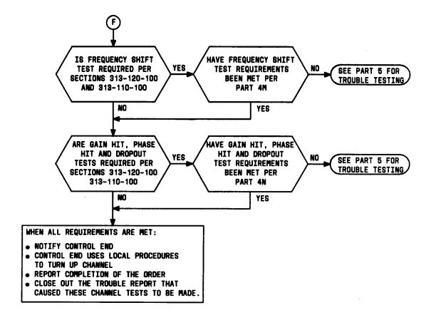
Flowchart 1—Required Preservice and Trouble Tests (Sheet 7 of 7)
