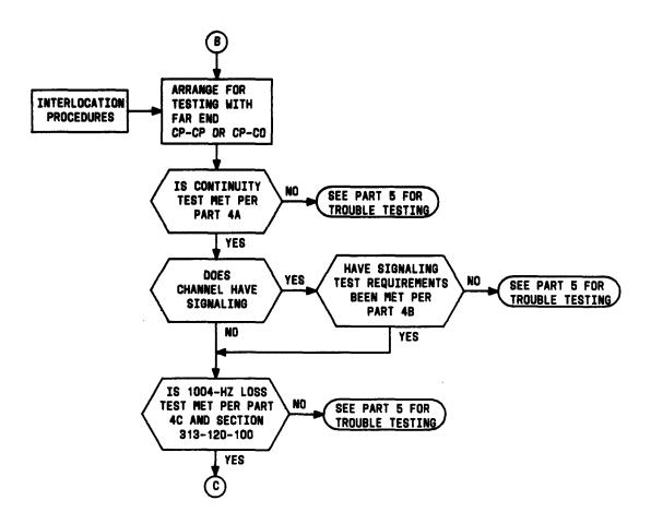
Flowchart 1—Required Preservice and Trouble Tests (Sheet 3 of 7)
