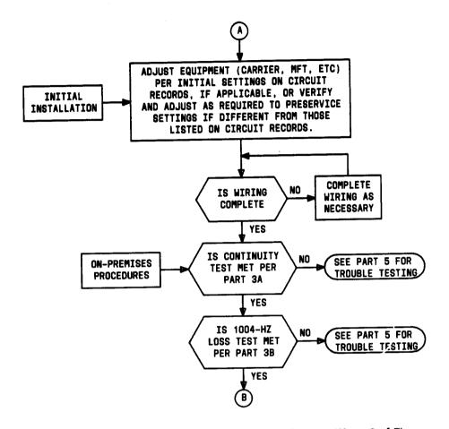
Flowchart 1—Required Preservice and Trouble Tests (Sheet 2 of 7)
