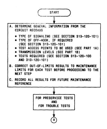
Flowchart 1—Required Preservice and Trouble Tests (Sheet 1 of 7)
