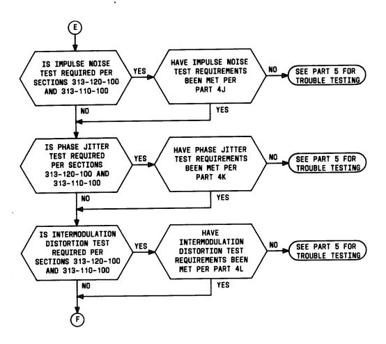
Flowchart 1—Required Preservice and Trouble Tests (Sheet 6 of 7)
