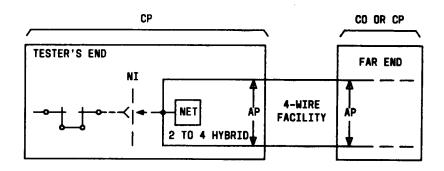
Fig. 1—2-Wire to 4-Wire Conversion at Tester's End
