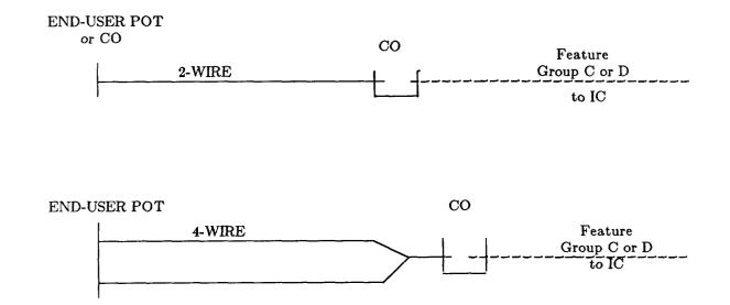
Figure 15. Typical WATS Access Line Configurations
