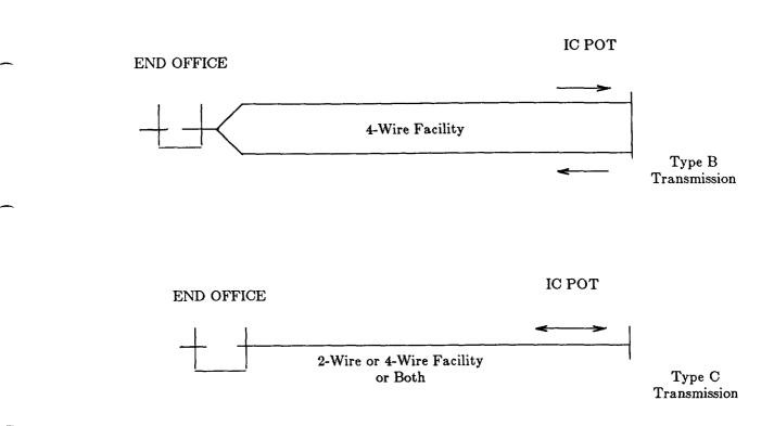
Figure 16. Typical Feature Group A Configurations
