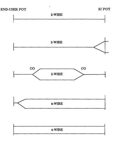
Figure 3. Typical VG1 Channel Configurations
