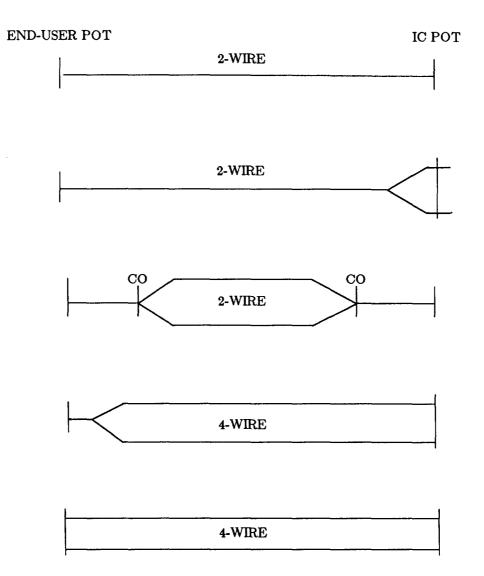
Figure 13. Typical VG11 Channel Configurations
