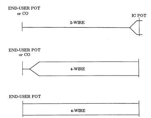
Figure 9. Typical VG7 Channel Configurations
