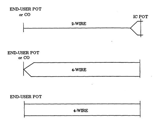
Figure 5. Typical VG3 Channel Configurations
