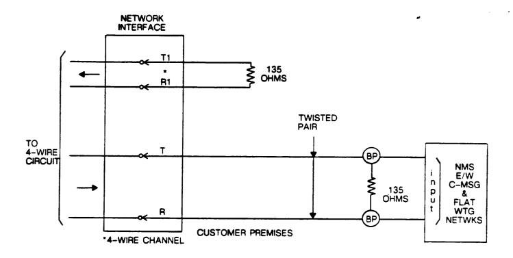
Figure 2. Test Connection For Noise Measurements
