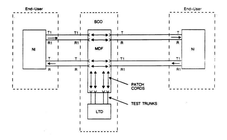
Figure 1. Test Access to a Local Area Data Channel Routed Through the SCO
