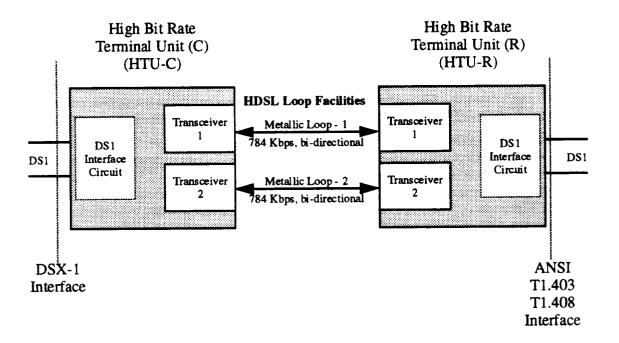
Figure 1.1 High Bit Rate Digital Subscriber Line (HDSL) System
