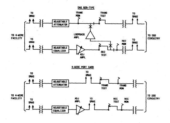
Fig. 10—Test Lines to Master Station Access Leads on DAS 829-Type and 4-Wire Ports
