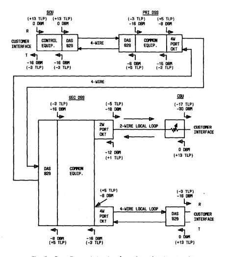
Fig. 5—Data Transmission Levels on 2- and 4-Wire Local Loops
