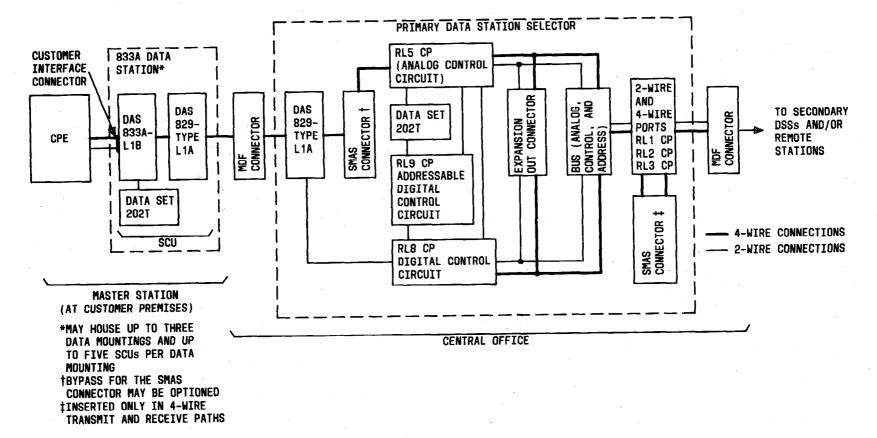
Fig. 4—Functional Block Diagram of Addressable Service Offering
