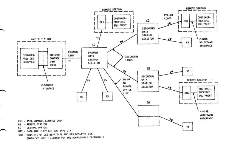
Fig. 1—Select-A-Station Service—Overall Block Diagram
