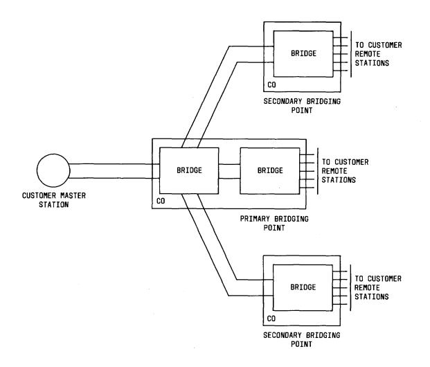
Fig. 1—Primary and Secondary Bridging Arrangement
