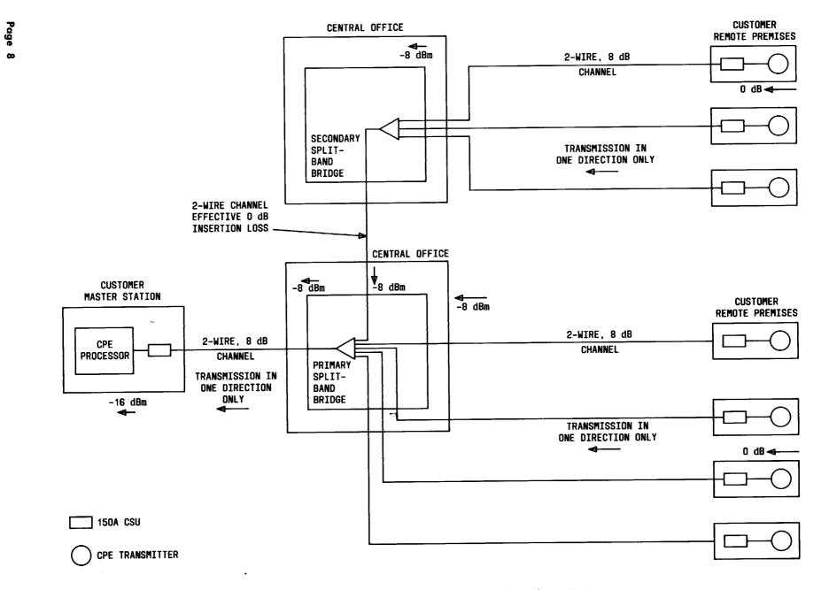
Fig. 5—Summation, Active Bridging Using Split-Band Bridging Equipment
