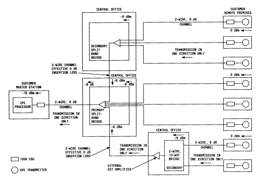
Fig. 7—Summation, Active Bridging Using A Combination of Split-Band and Passive Bridging Equipment
