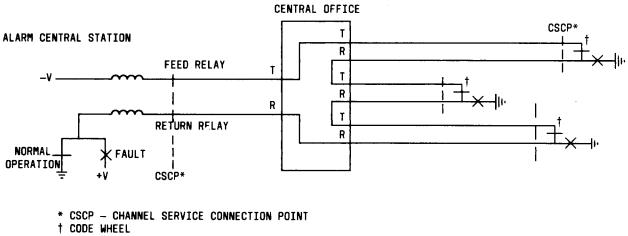
Fig. 1-Basic McCulloh Circuit Configuration
