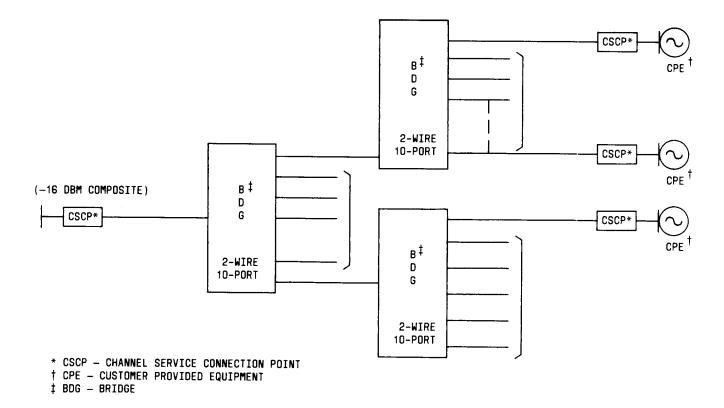
Fig. 8—Telemetry/Alarm Bridging Service, Summation
