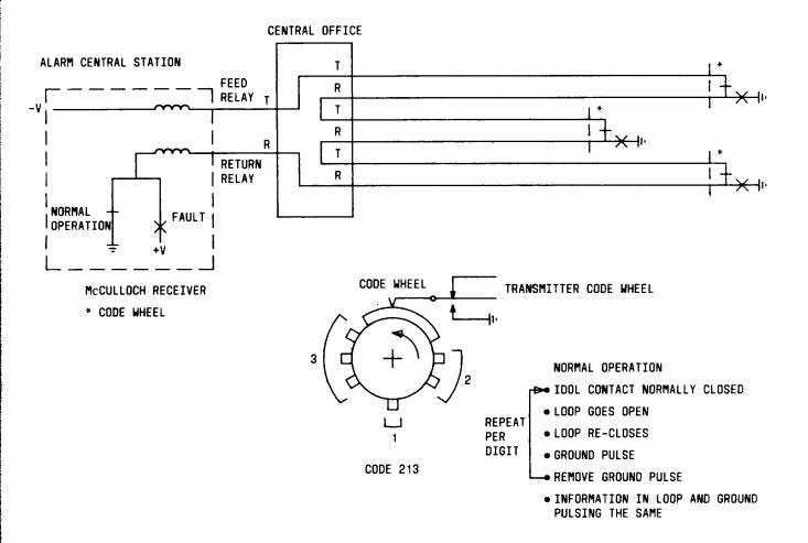
Fig. 5—Basic McCulloh Circuit Operation
