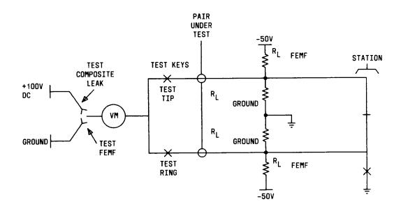
Fig. 3—Measurements for Foreign Voltage or Leakage to Ground
