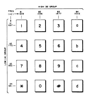
Fig. 7—TOUCH-TONE Button Designations and Frequency Assignments When Used With the 1A TTTLS
