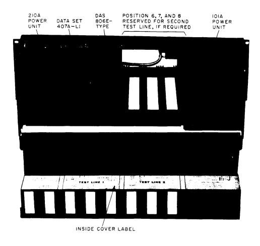
Fig. 1— 1A TTTLS—One Test Line Installed
