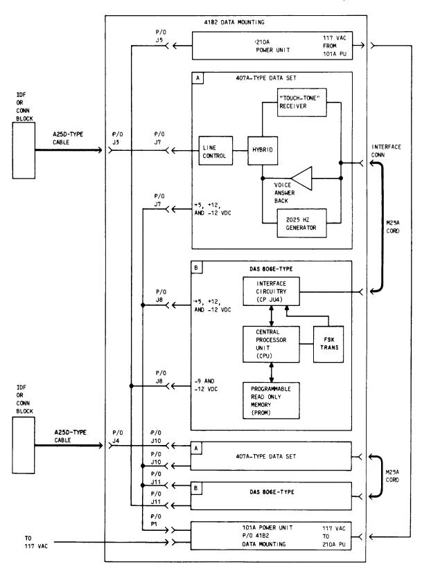
Fig. 6— Functional Arrangement—1A TTTLS—Typical
