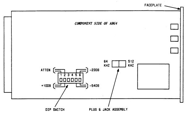
Fig. 18 - Location of Options for the AHG4 Timing Distributor
