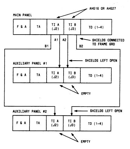
Fig. 24 - Cabling Diagram Showing Wiring Between Main and Auxiliary Panels
