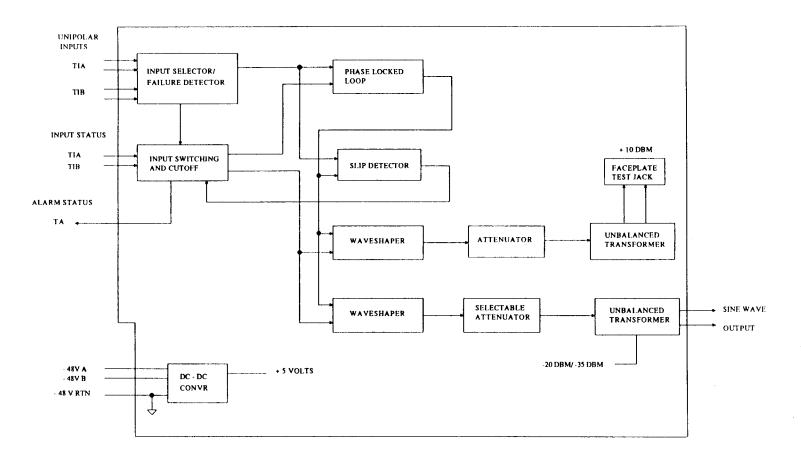
Fig. 19 - Block Diagram of AHG26 Timing Distributor
