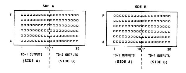
Fig. 5 - SDE() Terminal Block Assignments for DS-1 Outputs
