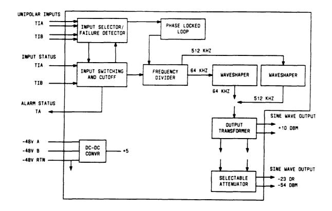
Fig. 16 - Block Diagram of Timing Distributor (AHG4)
