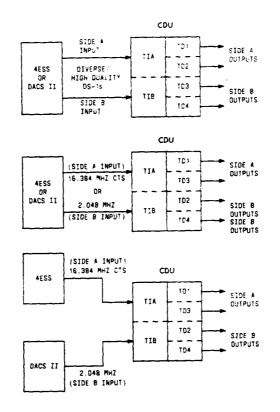
Fig. 3 - Typical Clock Distribution Unit Applications
