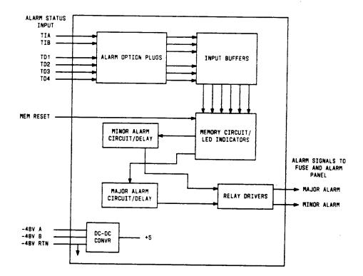
Fig. 22 - Block Diagram of Timing Alarm (AHG1)
