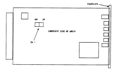
Fig. 9 - Location of Options on the AHG16 Timing Interface Circuit Pack
