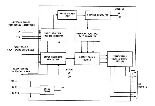
Fig. 13 - Block Diagram of the AHG25 Timing Distributor
