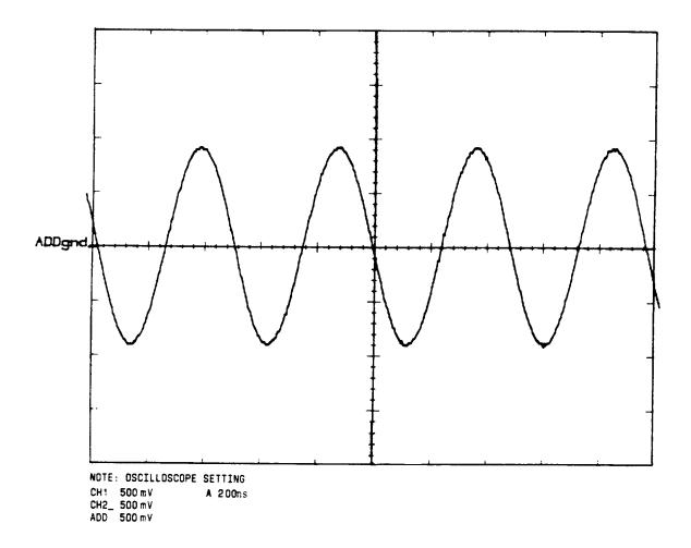
Fig. 20 - AHG26 TD Faceplate Jack (2.048 MHz at  $\pm 10~dBm)$
