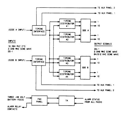
Fig. 4 - Block Diagram of Clock Distribution Unit
