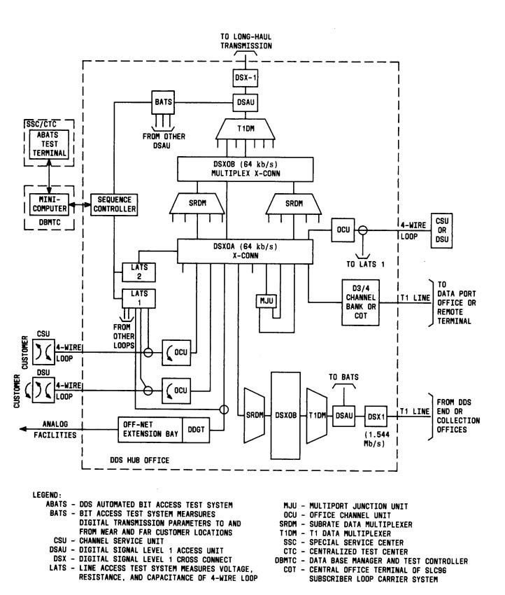
Fig. 3—DDS Hub Office Using ABATS/ALATS
