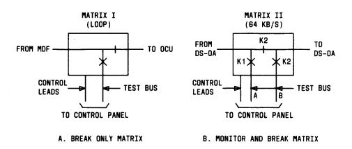
Fig. 5—Matrix Unit Configurations
