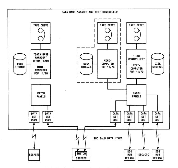
Fig. 2—Data Base Manager and Test Controller Configuration
