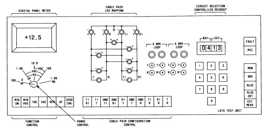
Fig. 6---Front View of LATS Control Panel
