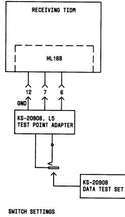
INPUT - LOGIC, FAR Counter - Ext Pulses Counter Mode - Reset Power - On
