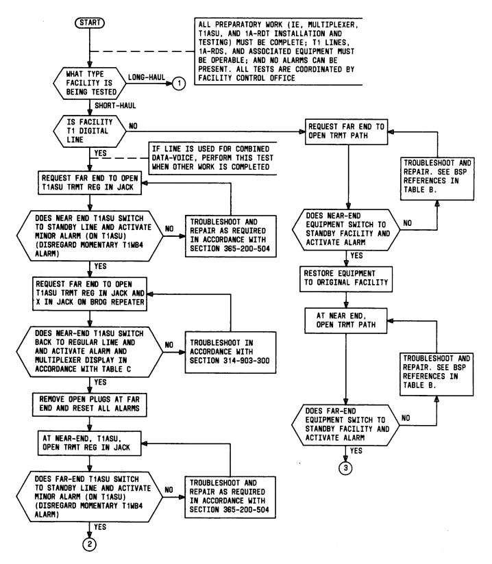
Fig. 4—#Facility Alarm Verification Test (Sheet 1 of 2) 4
