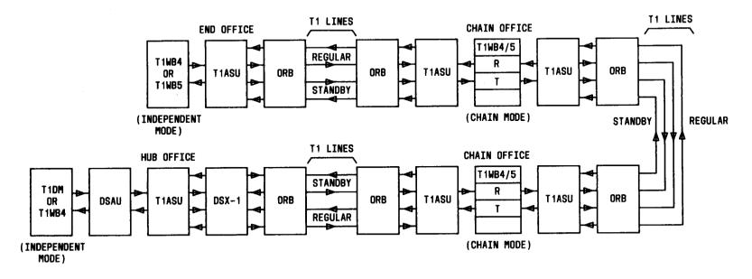
C. CHAIN OPERATION (DATA ONLY) WITH EITHER TIDM OR TIWB4 AT HUB OFFICE
