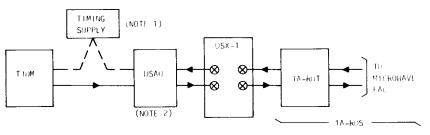
A. TERMINATING ARRANGEMENT WITH 1A-RDT IN HUB OFFICE
