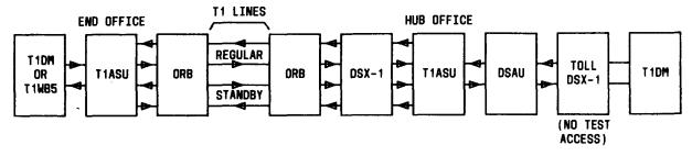
A. DIRECT LINE TERMINATING IN T1DMs OR T1WB5s (ALL DATA)
