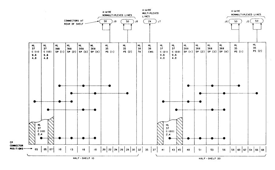
Fig. 3—♦Cable Connectors and Circuit Pack Interconnection♦
