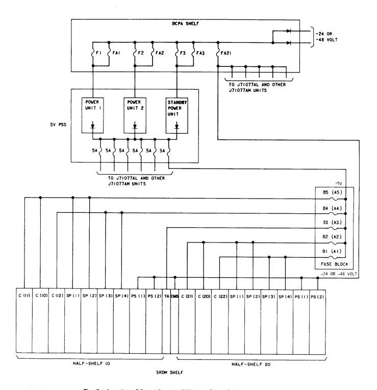
Fig. 2—Location of Fuses Serving SRDM and 5-Volt Power Supply Shelves
