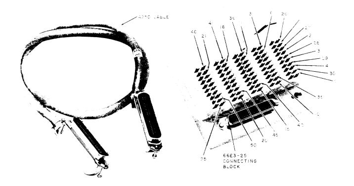
Fig. 5—A25D Double-Ended Connector Cable and 66E3-25 Connector Block With Terminal Locations
