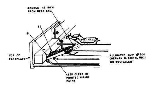
Fig. 1 — Temporary Modification of HL37 Common Logic Circuit Pack Using Alligator Clip to Disable Line Driver
