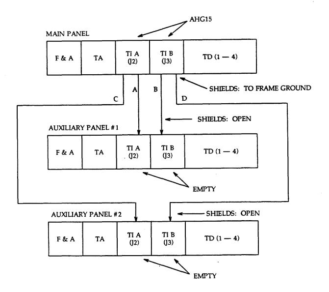
Figure 1-1. Cabling Diagram Showing Wiring Between Main and Auxiliary Panels Using the AHG15
