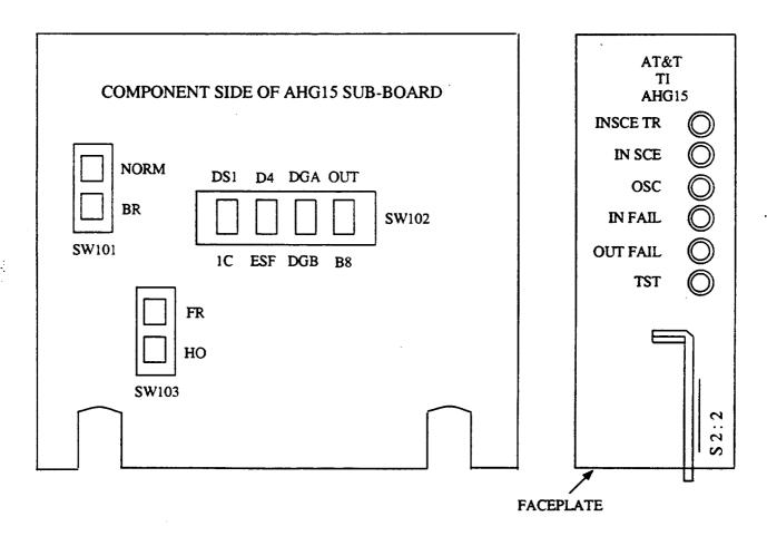
Figure 1-2. Location of Options on the Timing Interface Plug-In Unit, AHG15
