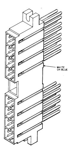
Fig. 6—Quad Terminal Block Assembly
