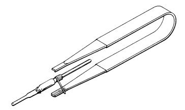
Fig. 5—Terminal Pin and Wire With Insertion Tool
