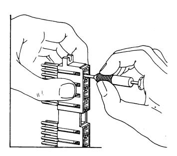
Fig. 7—Terminal Pin Extraction
