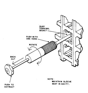
Fig. 4—Quad Terminal Pin Extraction
