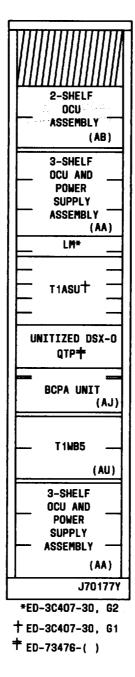
Fig. 6—11-Foot 6-Inch T1WB5 Local Office Bay Arrangement
