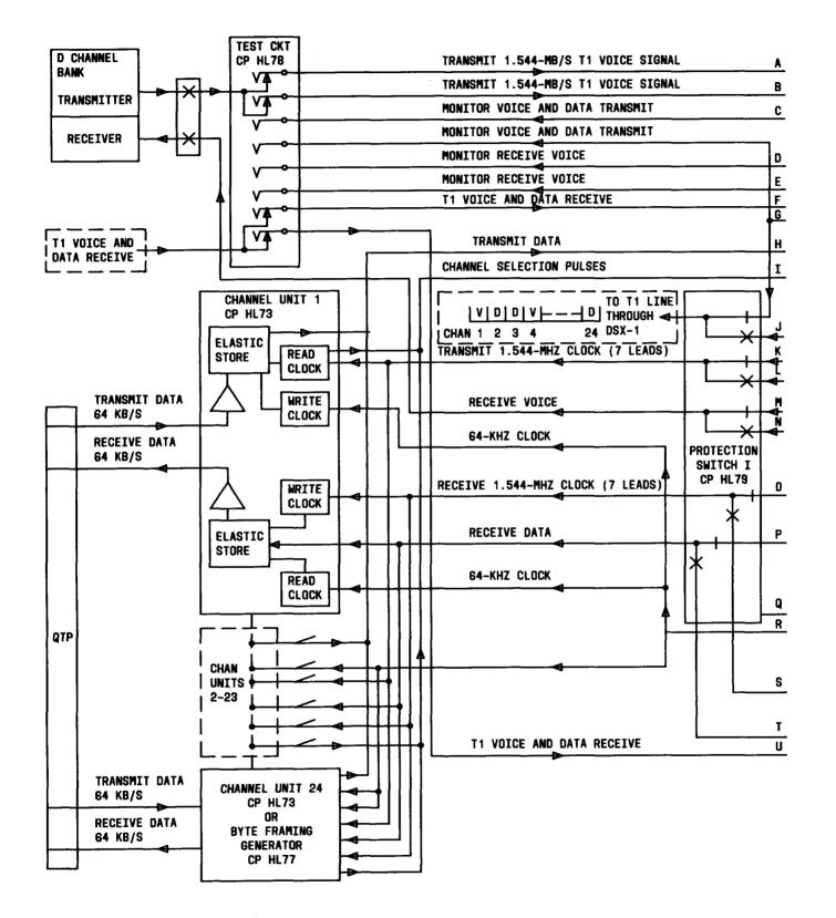
Fig. 4—\$T1WB5 Functional Block Diagram\$ (Sheet 1 of 3)
