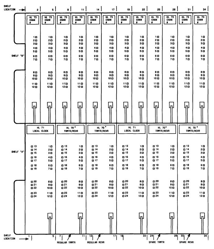
THE HL70C CAN BE USED TO REPLACE THE HL70 IN ALL CASES BUT THE HL70B OR HL70C IS REQUIRED IN THE TRANSMITTER REGULAR AND SPARE SLOTS WHEN A T1DM IS LOCATED AT THE DISTANT END. THE HL70C MUST BE USED FOR SECONDARY CHANNEL SERVICE.
