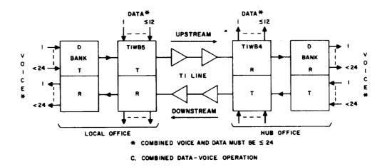
Fig. 3—T1WB5 Modes of Operation
