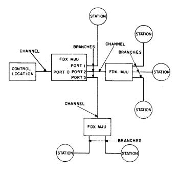
Fig. 1—Digital Data System Full-Duplex Multipoint Network
