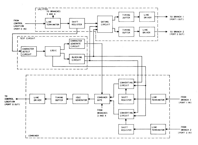
Fig. 10—Block Diagram of Full-Duplex Multipoint Junction Unit (HL68 CP)
