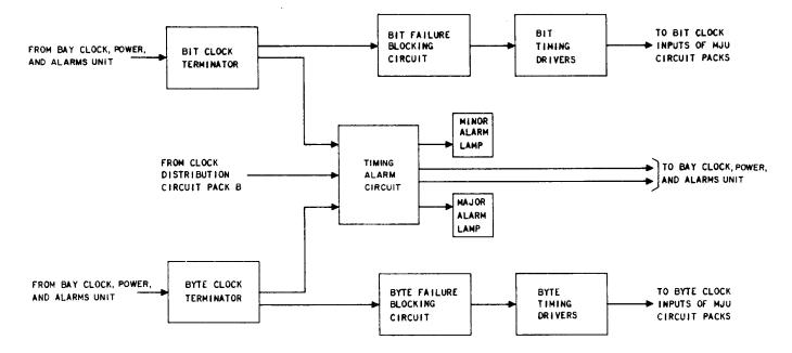
Fig. 11—Block Diagram of Clock Distribution Circuit Pack (HL69)
