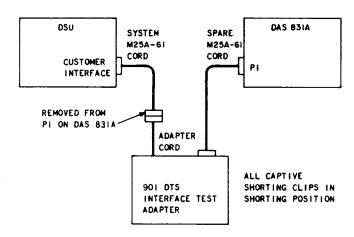
Fig. 6—Setup for DSU/DAS Interface Test Using Interface
