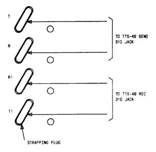
Fig. 9—171C Adapter—Test Connections
