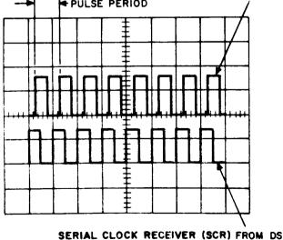
Fig. 8—Timing Phase Test—Oscilloscope Presentation
