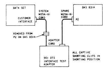
Fig. 4—Setup for Data Set/DAS Interface Test Using Interface Test Adapter
