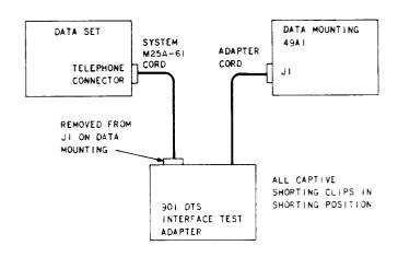
Fig. 2—Setup for Power Supply Test Using Interface Test
