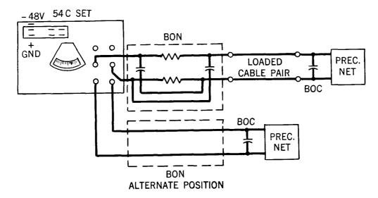
Circuit for Return-Loss Measurements
