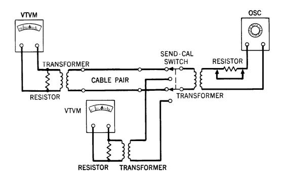
Circuit for Transmission-Loss Measurements
