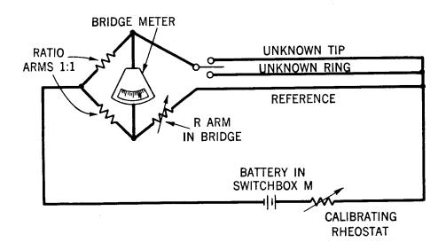
Circuit for Resistance Measurements
