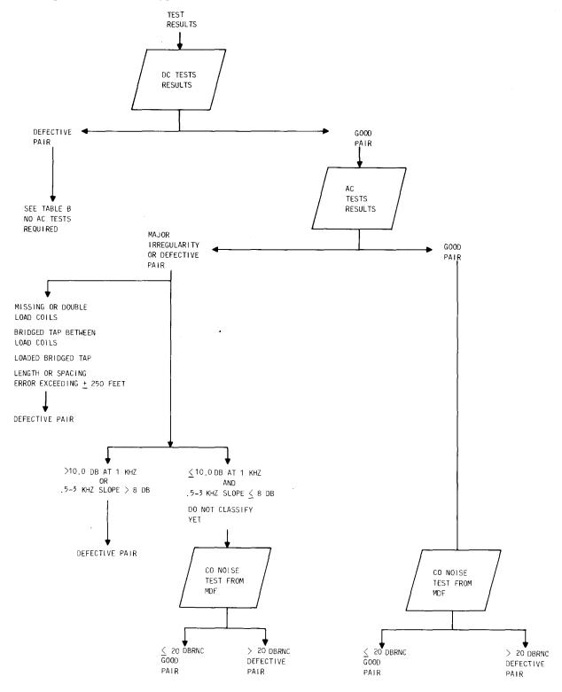
Fig. 1—Flowchart for Short Loaded Cables
