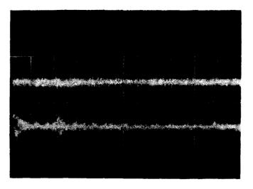
Fig. 1-Random Noise and Telephone Channel Noise
