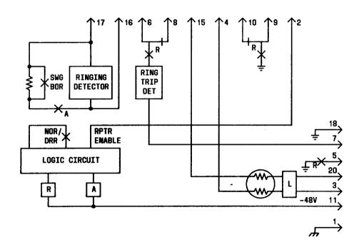
Fig. 1—Block Diagram of the J99343AK
