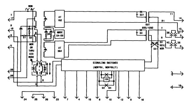
Fig. 1-J99343BF-1, L1 Block Diagram
