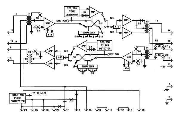
Fig. 1—J99343SF-1, L1 Block Diagram
