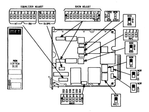
Fig. 2-J99343RA-1, L4 Component Layout
