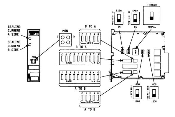
Fig. 2—Illustration of J99343SD Showing Location of Switches and Sealing-Current Indicators
