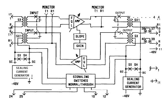
Fig. 1 -Block Diagram of J99343SD Unit
