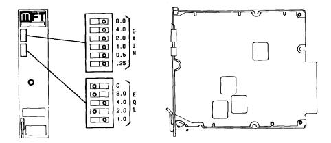
Fig. 2-J99343GR CFU - Component Layout
