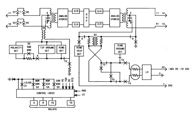
Fig. 1-J99343GS CFU-Block Diagram
