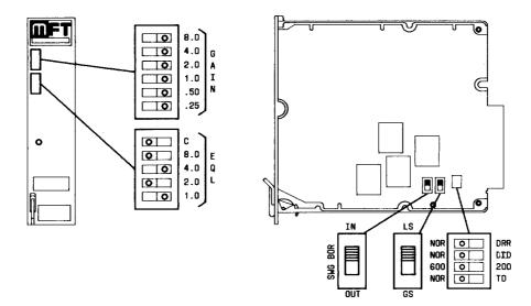
Fig. 2—J99343GS CFU—Switch Layout
