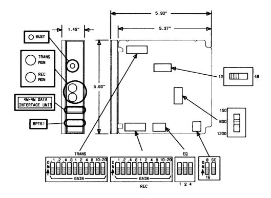
Fig. 2-BPT61 Unit Controls and Faceplate
