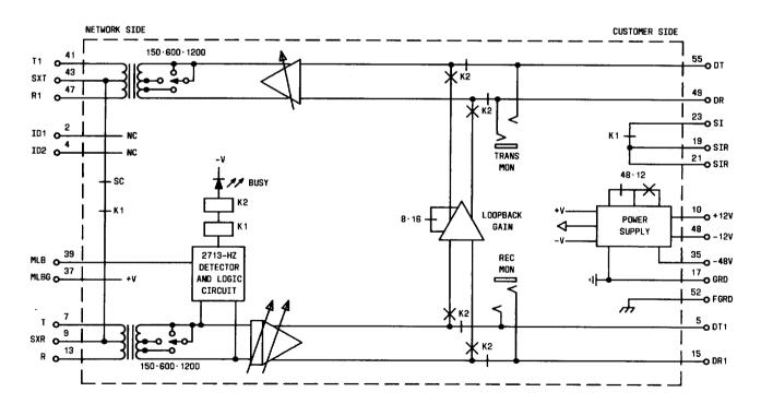
Fig. 1—Block Diagram of BPT61
