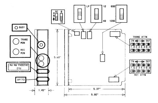
Fig. 2—BPT73 Unit Controls and Faceplate
