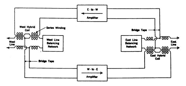
Fig. 1 — Hybrid Coil Type Repeater
