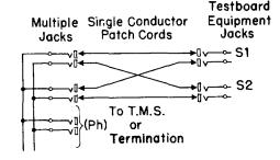
Fig. 1 2-Wire Equipment Jack Arrangements
