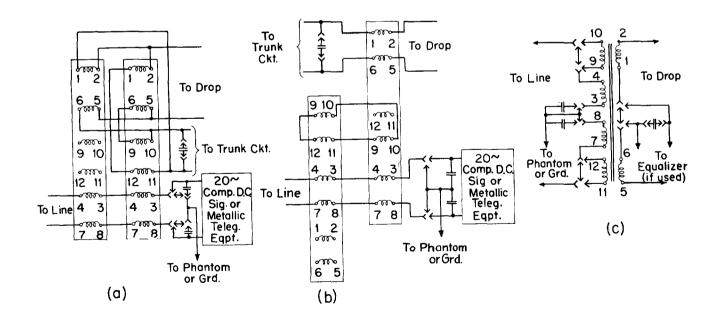
Fig. 5 - Transformer Arrangements for Non-repeatered Terminal
