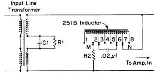
Fig. 6 - Equalizer for 4-Wire Circuits
