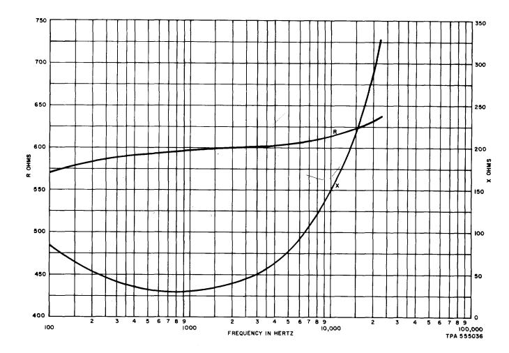
Fig. 4—F58122 Amplifier—Input Impedance—600-Ohm Termination
