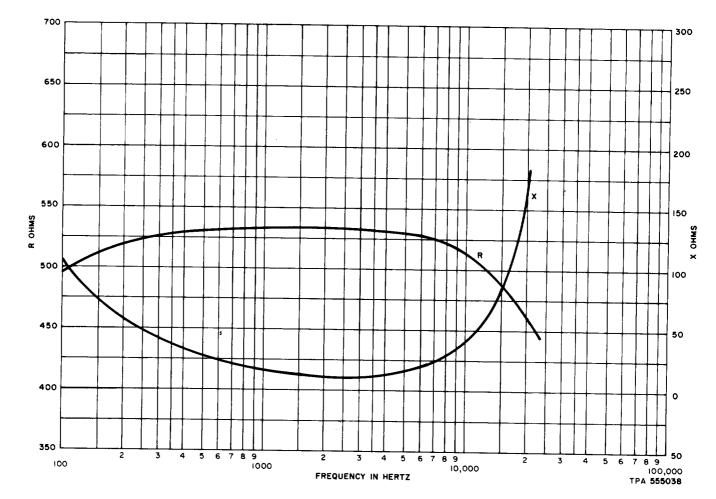
Fig. 6—F58122 Amplifier—Output Impedance—600-Ohm Termination
