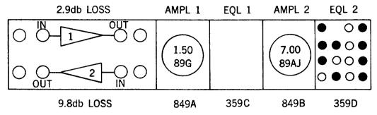
Fig. 5b – Example of 44V4 with Networks Instead of Amplifiers
