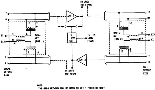
THE BASJ NETWORK MAY BE USED IN NET 1 POSITION ONLY WHEN THE ZG OPTION HAS BEEN WIRED PER SD 97047-01, ISSUE 23 OR LATER.
