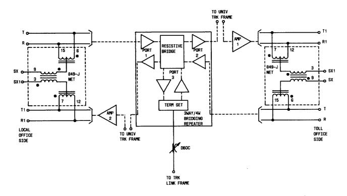
Fig. 4—Simplified Schematic of J99338F 4-Wire Bridging Repeater With 849J Networks
