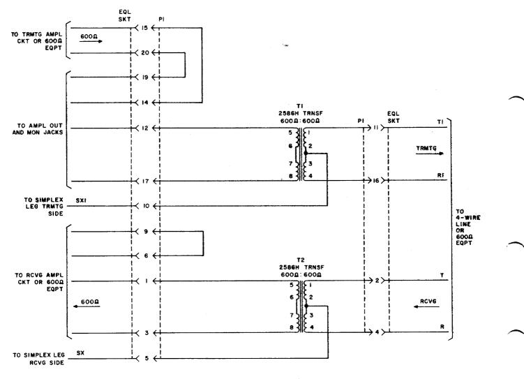
Fig. 2—359F Equalizer—Schematic and Typical Circuit Connections
