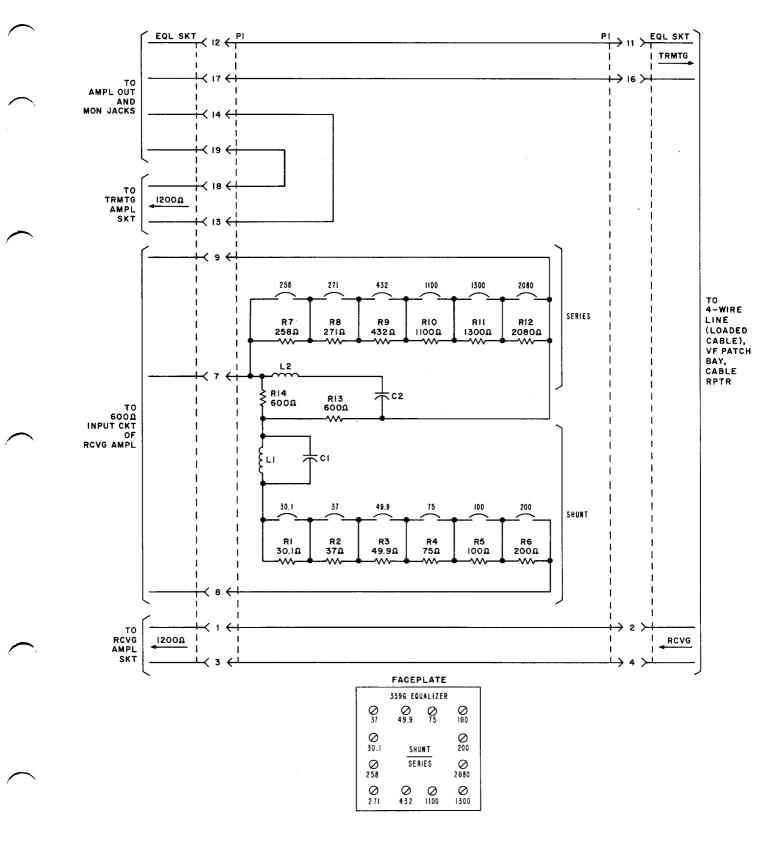
Fig. 2—359G Equalizer—Schematic—Typical Circuit Connections for 44V4B Repeater Associated With Data Trunk
