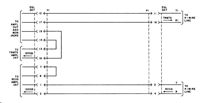
Fig. 2—359J Equalizer—Schematic and Typical Circuit Connections
