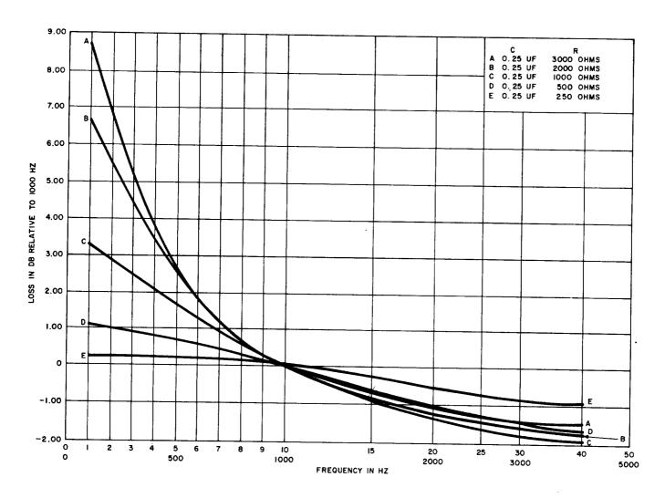
Fig. 4—359L Equalizer—Loss-Frequency Characteristics—Between 600 Ohms—Keeping C Constant and Varying R
