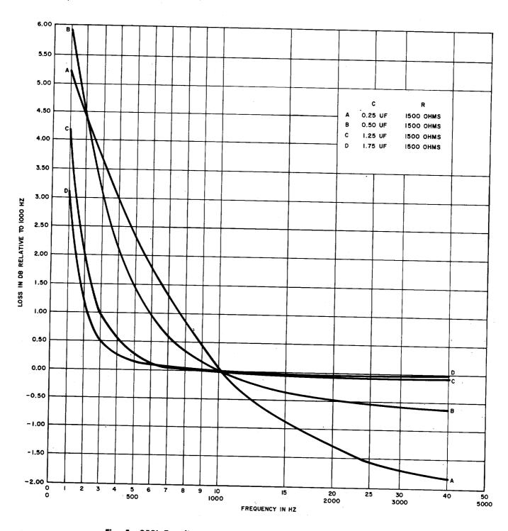
Fig. 5—359L Equalizer—Loss-Frequency Characteristics—Between 600 Ohms—Keeping R Constant and Varying C
