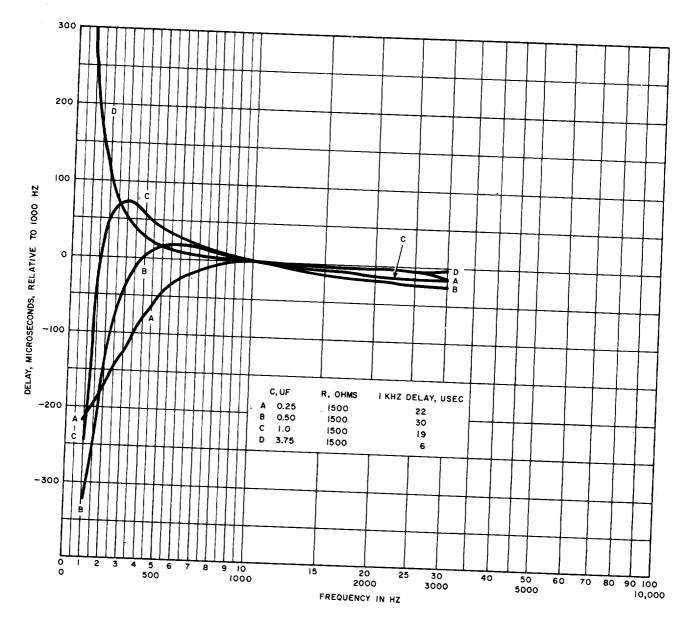
Fig. 7—359L Equalizer—Delay-Frequency Characteristics—Between 600 Ohms—Varying C for R=1500 Ohms
