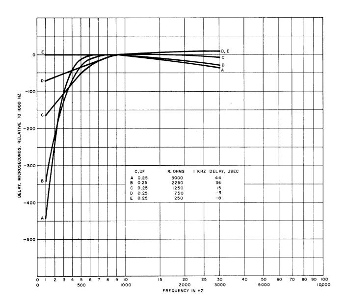
Fig. 6—359L Equalizer—Delay-Frequency Characteristics—Between 600 Ohms—Varying R for C=0.25  $\mu F$
