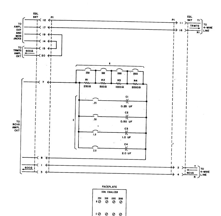
Fig. 3—359L Equalizer—Schematic and Typical Circuit Connections
