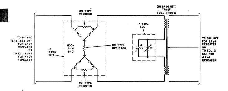
Fig. 2—359L Equalizer—General Circuit Configuration and Location in 849G
