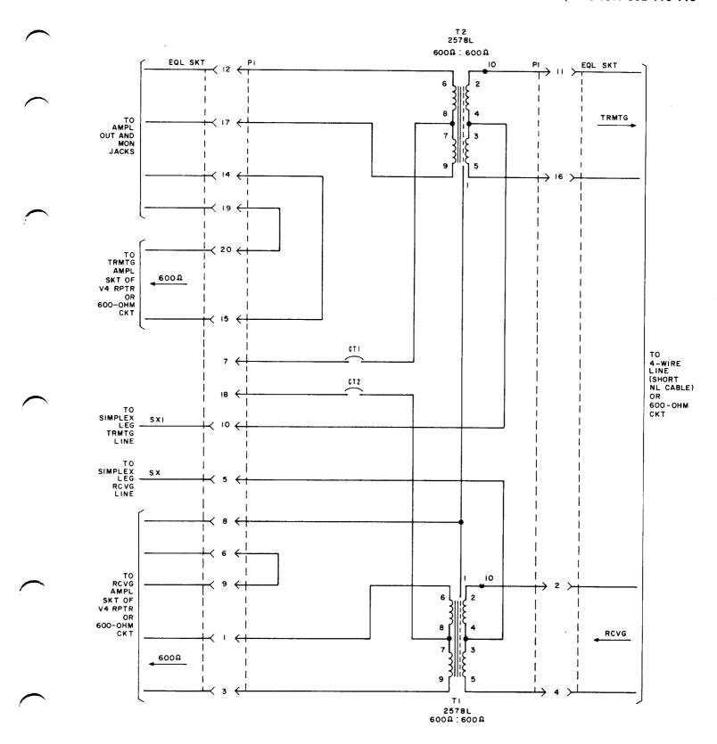
Fig. 2—359N Equalizer—Schematic and Typical Circuit Connections
