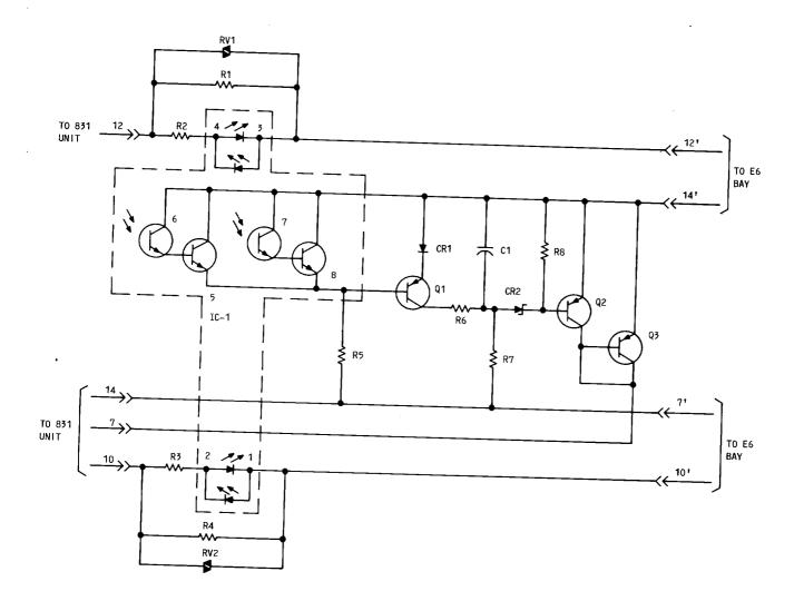
Fig. 3—Schematic Diagram of E6 Solid-State Disabler
