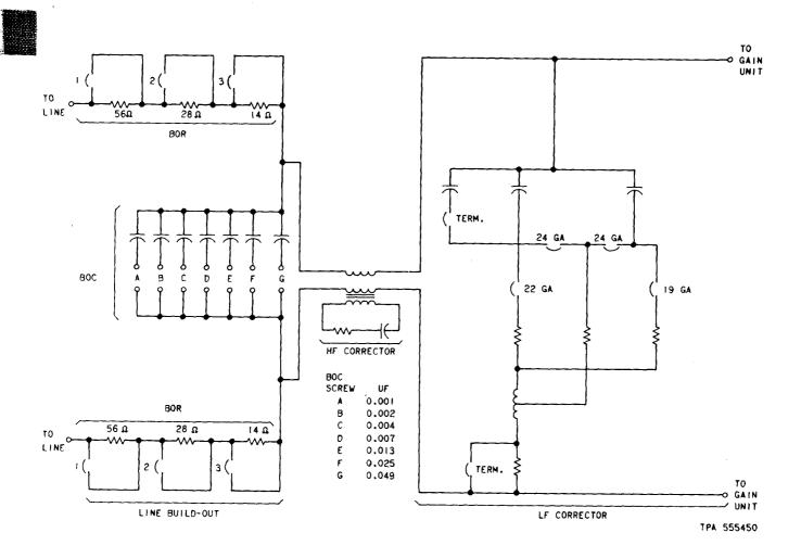
Fig. 2—830A Network—Schematic Diagram
