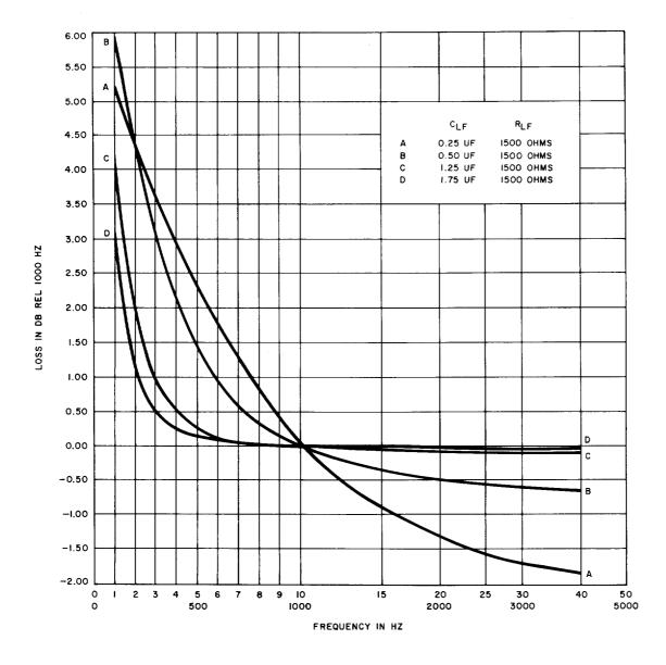
Fig. 5—4182C Network, Low-Frequency Section, Loss-Frequency Charcteristics Between 600-Ohm Impedances—Varying Cur For Ru Constant at 1500 Ohms
