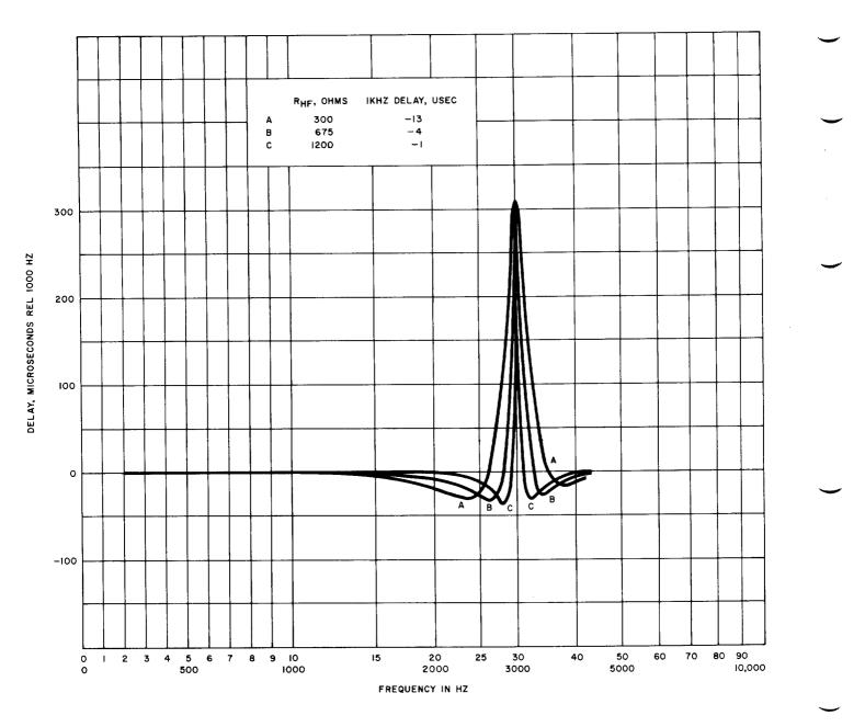
Fig. 9—4182C Network, High-Frequency Section, Delay-Frequency Characteristics Between 600-Ohm Impedances—At Various Settings of R<sub>HF</sub>
