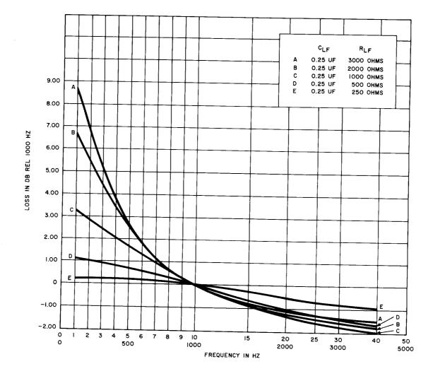
Fig. 4—4182C Network, Low-Frequency Section, Loss-Frequency Characteristics Between 600-Ohm Impedance—Varying Ruf For Cuf Constant at 0.25 μF
