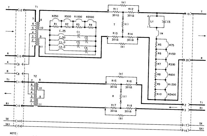
RESISTORS (a), (b),AND (c) ARE CONTAINED IN THE PLUG-IN 89-TYPE RESISTOR AND ARE NOT FURNISHED WITH THIS NETWORK.
