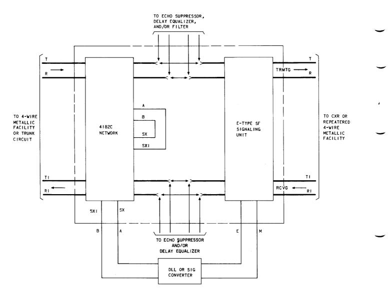
Fig. 11—4182C Network Used in VF Terminal Equipment Bay—Signal Conversion Required
