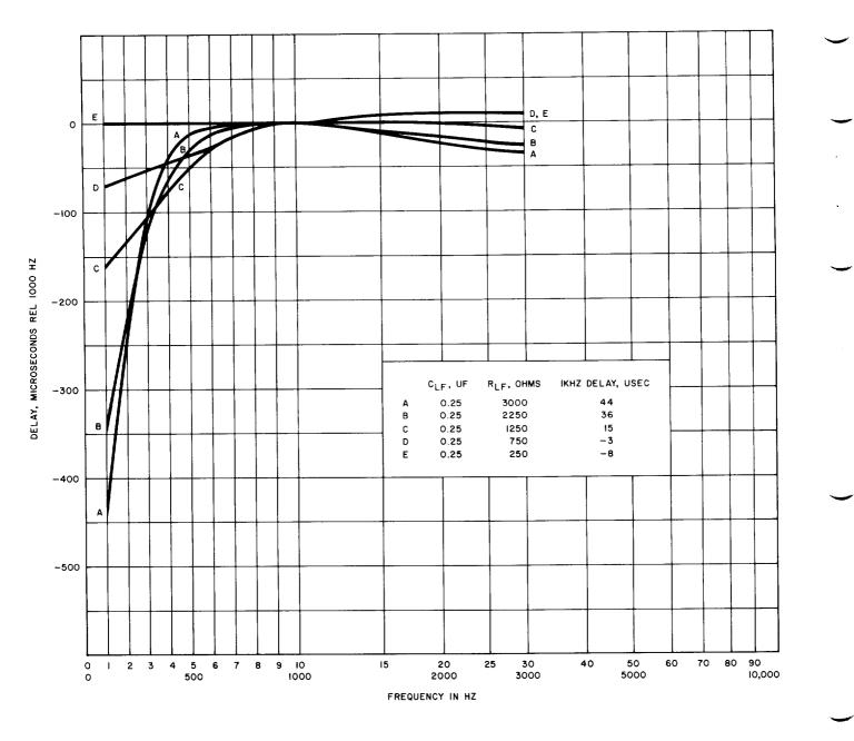
Fig. 7—4182C Network, Low-Frequency Section, Delay-Frequency Characteristics Between 600-Ohm Impedances— Varying RF for CF = 0.25  $\mu$ F
