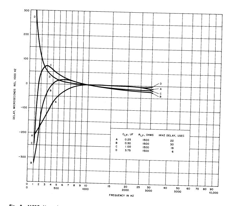
Fig. 8—4182C Network, Low-Frequency Section, Delay-Frequency Characteristics Between 600-Ohm Impedances— Varying C# For R# = 1500 Ohms
