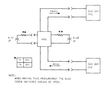
Fig. 4—Transhybrid Loss Measurement of 1P/1R Terminating Set
