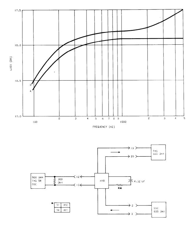
Fig. 3—1P/1R Terminating Set Transducer Characteristics
